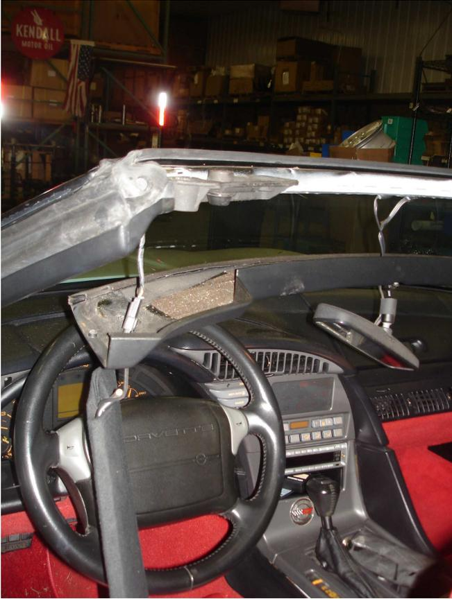
5. Go to roof and make sure front plate assembly on roof is loose enough to move by hand.
