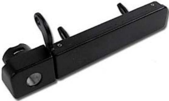
“The door handles are built with a very inexpensive metal, that get coated with a crinkle coat black finish to hide any imperfections. The metal is porous and not smooth enough to paint the body color,” Heinrich said. “There were a few sets of handles completed successfully using body-filler to smooth the surfaces, but it took too long to complete, and that concept was scratched. One car did leave the plant with the blue door handles, which was a convertible; it was Tom Daleworth’s car.”
