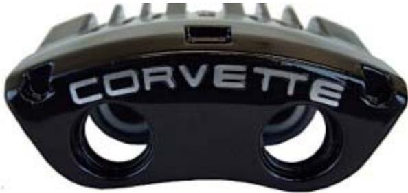
He continued, “The black brake calipers presented some challenges as well. The stock calipers were a real eyesore with the black wheels, and we couldn’t just leave them. Again, the casting was inexpensive which created a lot of issues when it came to painting. The provider agreed to use a different metal which ultimately resulted in a caliper that was much stronger and heat resistant. These calipers were also used on the Camaro and Firebird in 1997.”
